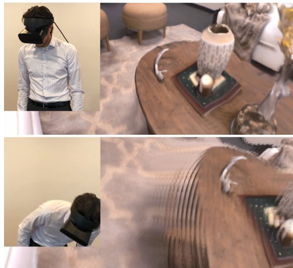
Fig. 13. Limitation: Using our system within a VR headset allows large motions away from the center of the MSI, exposing the layer structure of the representation ( bottom ).
