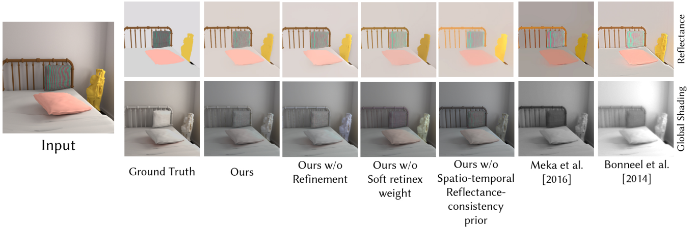
Fig. 18. Ablation study and qualitative comparisons on the SYNTHETICROOM sequence. Without the base color refinement, our approach incorrectly estimates blue illumination on the statue, the bedpost and the cushion. Without the soft-Retinex weighted monochromatic prior, the illumination incorrectly contains color across all the objects in the scene. Without the spatiotemporal prior, the reflectance estimate is inconsistent across uniform reflectance regions, such as the wall and the bedspread. Our result with the complete energy gives a more accurate decomposition that is closer to the ground truth. We accurately decompose the illumination from the pink cushion and within the yellow statue into the illumination layer, while the other intrinsic video decomposition methods incorrectly bake the color spill into the reflectance layer.
