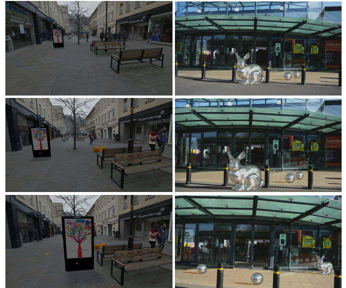
Figure 2: Scenes used to test the accuracy of synchronisation and compositing. Inserted CG elements include a poster stand (left) and a reflective bunny and two balls (right). Single frames extracted from the final composite sequence show that CG elements stay fixed in their places in the scene when the camera moves (first two rows). The video playback can be paused at any frame, and the inserted CG elements can be moved or changed using keyboard shortcuts (bottom row).
